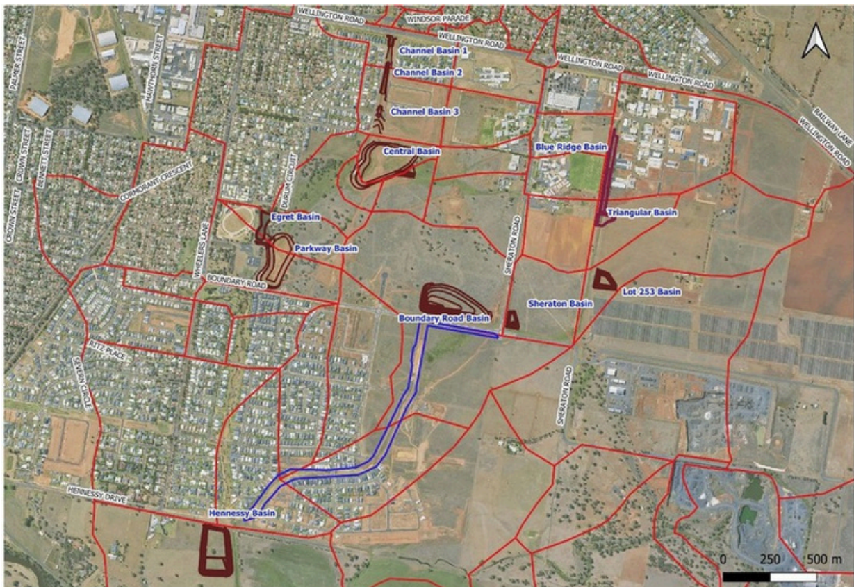
Figure 4 2024 Keswick Estate Trunk Drainage Scheme
